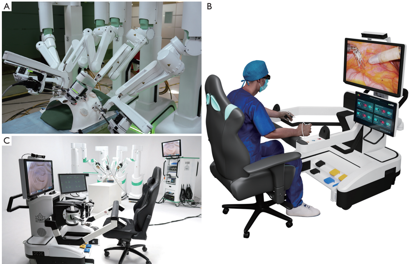
Figure 5 The SSI Mantra Surgical Robotic System courtesy of SS Innovations. (A) Arm carts, (B) surgeon command centre, (C) the SSI Mantra set-up.
