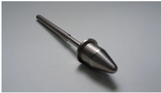
Figure 1 The original device. It has changeable cylinders with different diameters.
