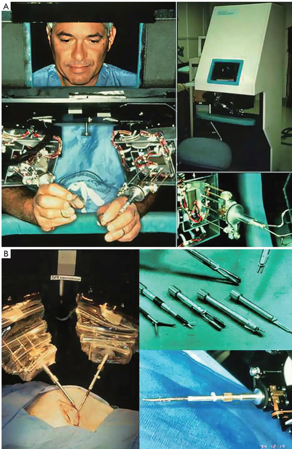
**Figure 6** The first surgical robot prototype. (A) Green telepresence surgeon's workstation with hand controls—Stanford Research Institute 1994. (B) Exchangeable end-effector surgical instruments. The figure is reproduced with permission from the *Journal of Laparoscopic Surgery and Society of Laparoscopic and Robotic Surgeon*.
