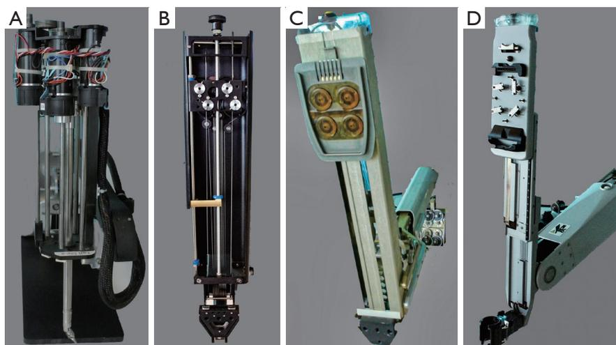
**Figure 9** Intuitive surgical instrument arm development. (A) Lenny the first prototype; (B) Mona—the first prototype used for clinical studies; (C) the first daVinci commercial arm; (D) daVinci S and Si commercial arms.
